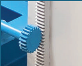
4 side rack Pinon Working platen insure uniform pressure increase life of cylinder
